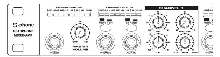
MASTER VOLUME – OFF CHANNEL 1 MUTE SWITCH – OUT CHANNEL 1 ST/2CH SWITCH – OUT CHANNEL 1 HIGH FREQUENCY – 0 CHANNEL 1 LOW FREQUENCY – 0
